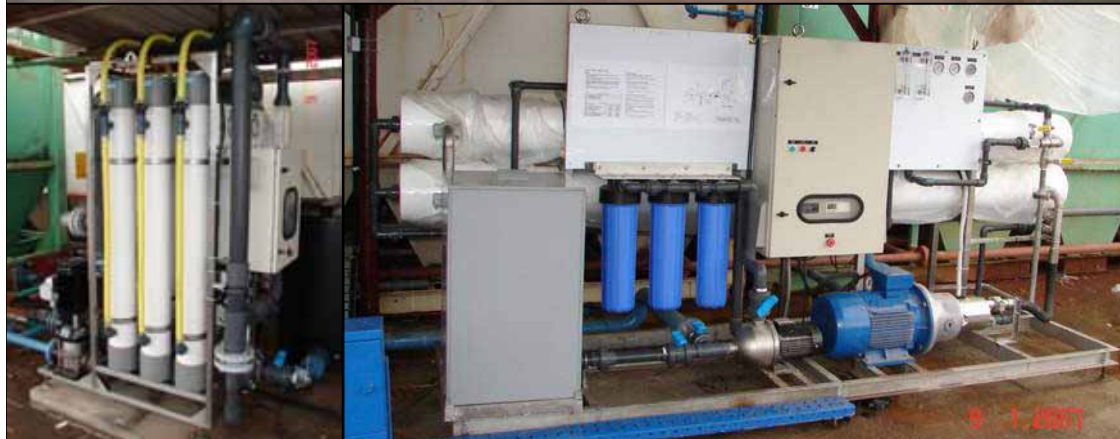
MU06-8 AND 6 SWRO ELEMENTS IN 2 VESSELS
