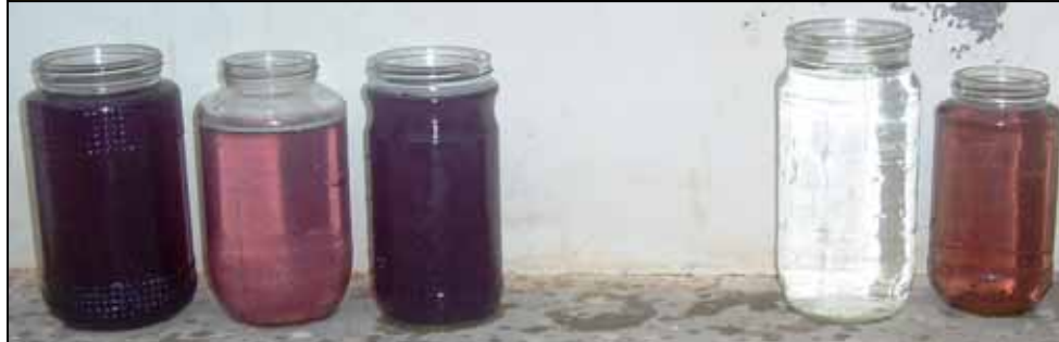
UF Feed Permeate Backflush RO Permeate Reject
